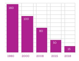
Pillard Burners NOx emissions improvement since 1980 in mg/Nm3 3%O2dry in gas firing
