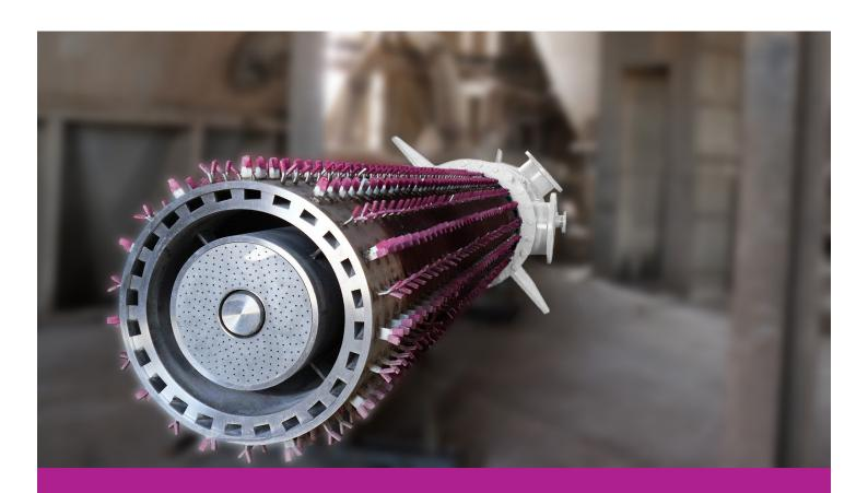
Tailor-designed to suit any precalciner type, firing gaseous, liquid and solid fuels
