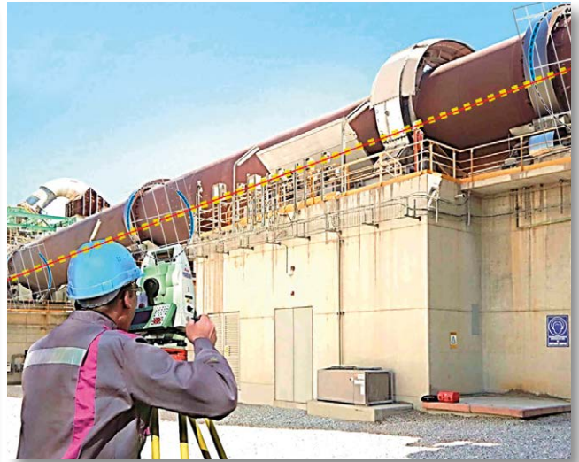
Figure 7: Rotary kiln alignment control
