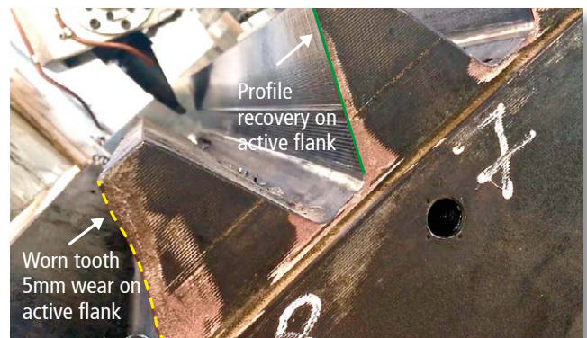
Figure 2: Machining in progress on a rotary kiln girth gear (228 teeth, modulus 28, width 690 mm)
