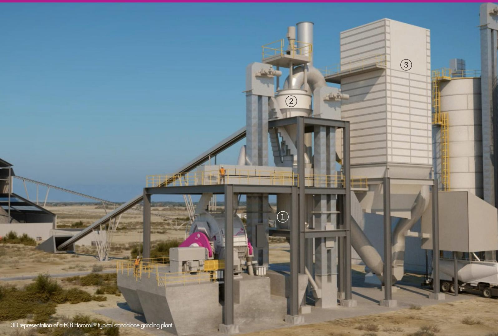
3D representation of a FCB Horomill® typical standalone grinding plant
