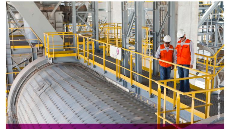
The FCB B-mill has been designed to be par<mark>ticular</mark>ly suitable for grinding high fineness products, highly abrasive materials, and solid fuels
