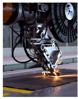
Dry fiber deposition - Wing of the future project - Madras line (IRT Jules Verne)
