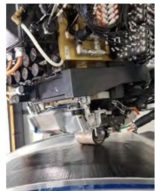
Process control using on-board optical coherence tomography
