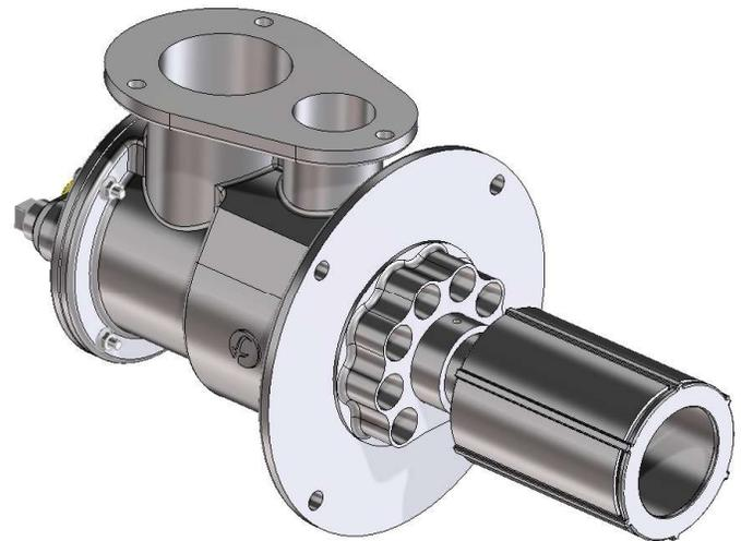
The durability of the Evenglow family is retained for the Evenglow LNx including high alloy cast flame retainer and sturdy cast iron throughout. Evenglow LNx burners include a built-in V-port fuel adjustment plug (ambient air only), multiple observation ports, a flanged air connection, and a gas connection that can be rotated in 90° increments. Flame ignition is accomplished with the included direct spark igniter. Flame monitoring is possible by ultraviolet flame detection (sold separately).
