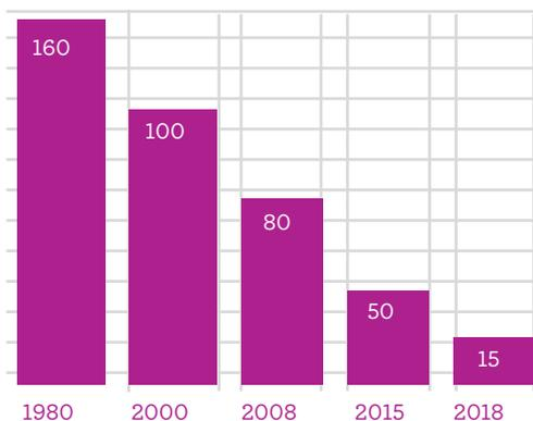
Pillard Burners NOx emissions improvement since 1980 in mg/Nm<sup>3</sup> 3%O<sub>2</sub>dry in gas firing
