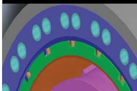
Figure 4: 3D model of the burner tip including the axial air inserts
