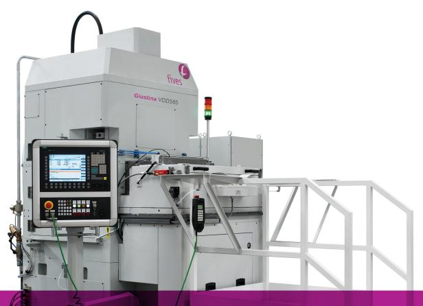
Vertical Double Disc grinder with 3-block cast iron box type framing for superior machine rigidity
