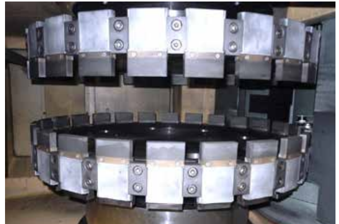
48 CBN or diamond segments (24 segments for each wheel)
