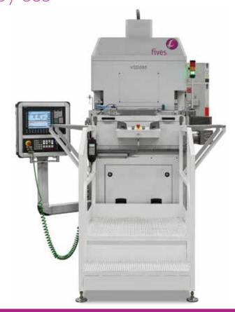
Vertical single disc grinder with an ID/OD clamping system, developed for the processing of sun gears
