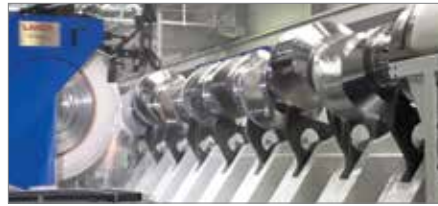
Grinding of pins on 6,500 mm crankshaft
