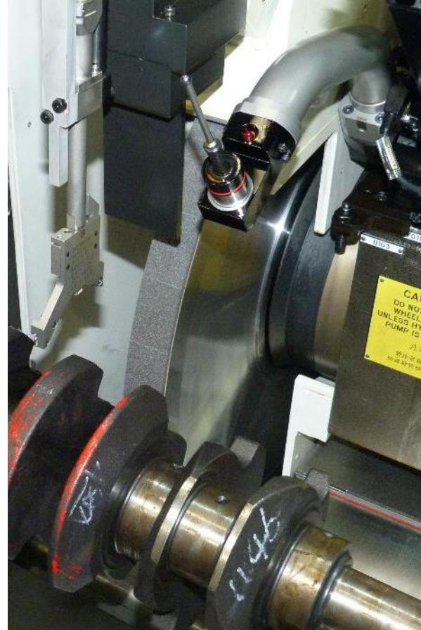
Finish grinding on mains & pins, including sidewalls and radii
