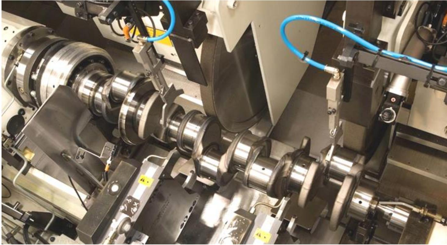
Finish grinding intake, exhaust cam lobes and injectors
