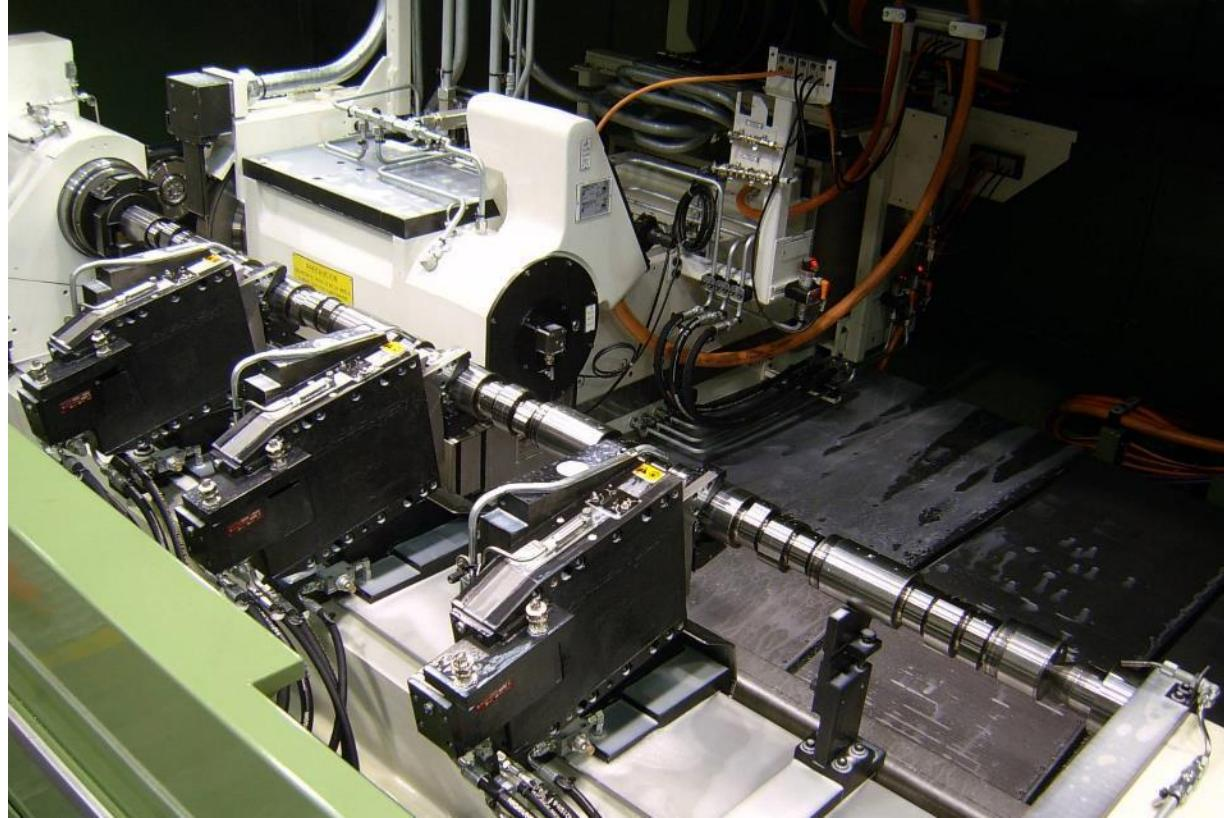
Semi finish and finish grind cam lobes on various shafts
