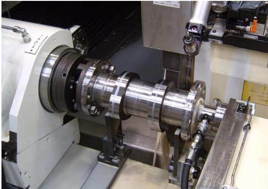
Finish grind mains & pins including sidewalls & radii
