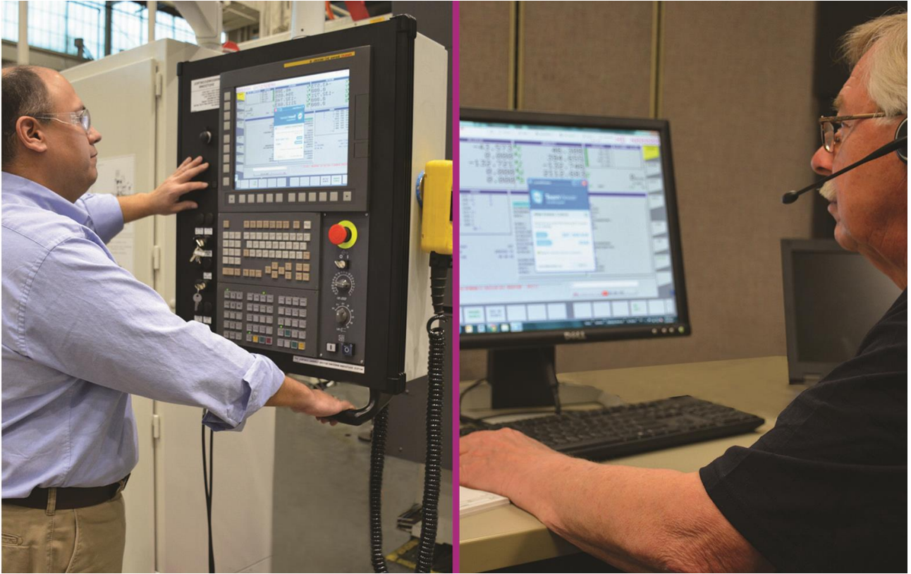
Fives Machining Systems (Diagnostic Communication System (DCS) connects machines in the field to Fives technicians
