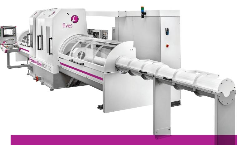
The Forest-Liné MGP™ 150 high-speed machining center is adapted to short and medium parts and is dedicated to the aerospace industry. It has been developed to perform both drilling, milling, chamfering, routing and end-machining operations on aluminum bars.
