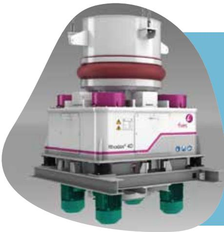
FCB Rhodax®'s selective material bed compression grinding process optimally releases the three components making up concrete - aggregates, sand (0.125-2 mm) and cement paste (0-0.125 mm), which will then be separated and retrieved.
