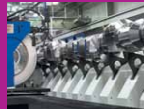
Page 42 • Crankshaft being grinded by a Landis machine
