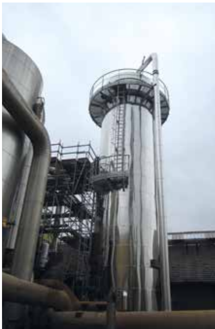
The Cail & Fletcher falling film evaporator guarantees optimized distribution of the juice
