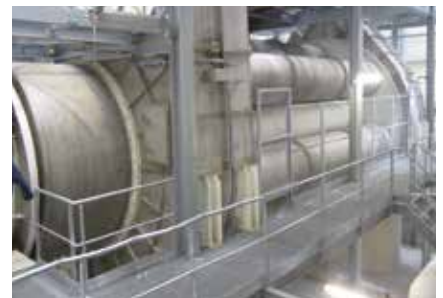
The Cail & Fletcher multitube dryer/cooler preserves crystal quality
