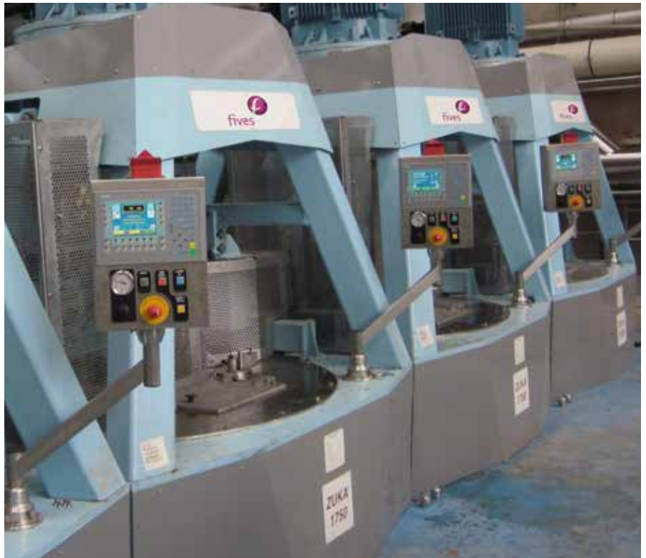
The Cail & Fletcher ZUKA® enables a 30% increase in capacity thanks to the double discharger
